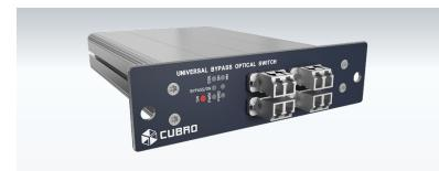
The single link Cubro Bypass for 1,10 & 100 Gbit single mode is realized with two MEMS optical switches. The switching mechanism offers the reliability of a solid state device. The optical switch is a latched version, this means it needs only power during switching operation. Even when power fails the optical switch stays in the programmed state.
