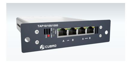
The Cubro 10/100/1000 Copper TAP allows the uninterrupted passage of full duplex data over standard Category 5/6 copper network cable. Featuring auto negotiating between 10Mbps, 100Mbps and 1000Mbps, this TAP duplicates the network signals, including any existing physical errors to the transmit-only monitoring ports.
