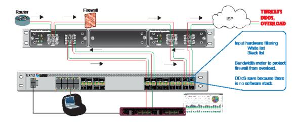
A bypass is a hardware device that provides a fail-safe access port for an in-line active security appliance. The EX12 monitors the health of the active in-line appliance by sending heartbeat packets through the security appliance and detecting them after they have passed through the device. If the security appliance fails then the heartbeat will not be detected and the EX12 can either reroute the traffic around the failed security appliance or reroute the traffic through a spare standby unit.
