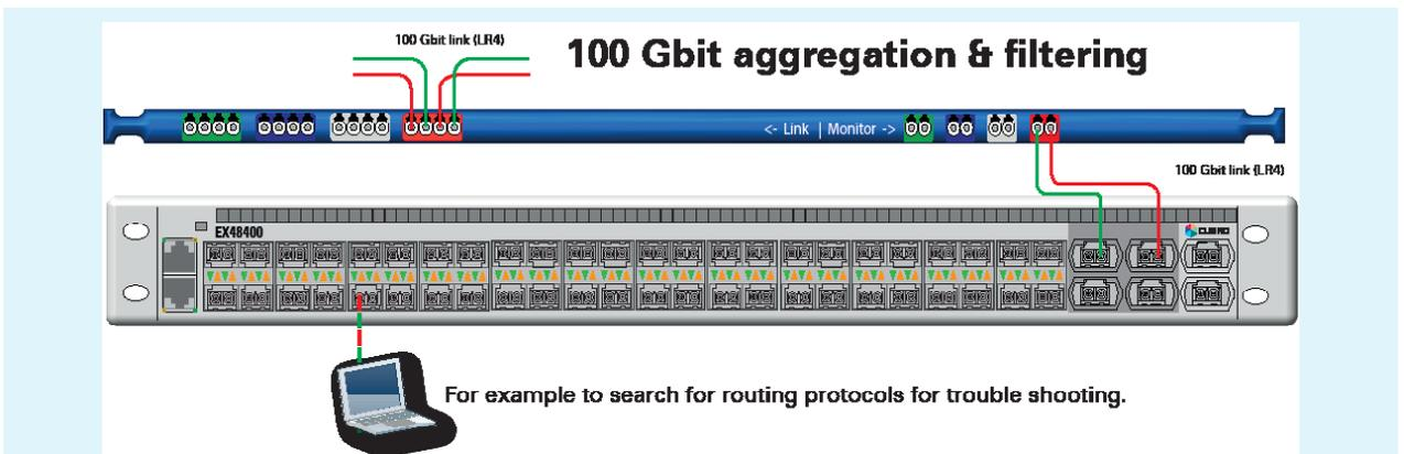
The Sessionmaster EXA32100 supports 4000 filters that can classify traffic. These filters can be used to redirect a selected part of the traffic to a low bandwidth monitoring tool, such as a 10G packet analyzer to troubleshoot an issue on a 100 Gbit link (such as a routing problem).
