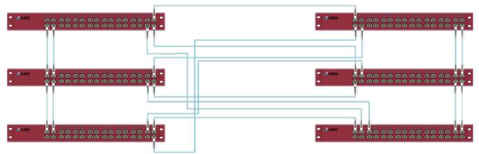
In this application 6 x EXA32100s are connected to a fully meshed cross connect with 162 available 100 Gbps ports (27 available ports per device). The interconnection between the devices can be done with one link or more depending on the bandwidth that is needed.
