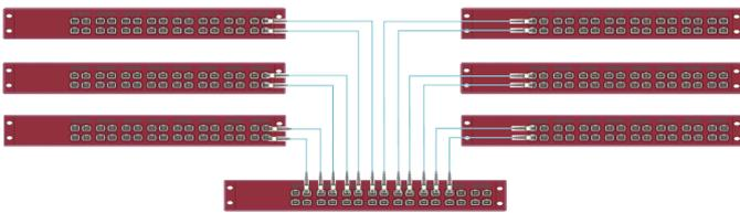
In this application 6 x EXA32100s are connected to a central unit with 186 available 100 Gbps ports (31 available ports per device).
