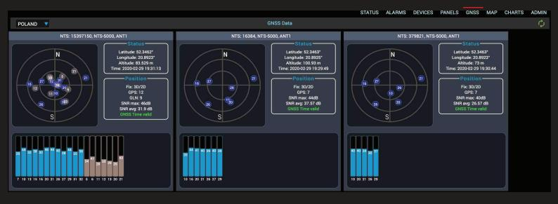
Each server's antenna is traceable individually. But you can also group receivers on one screen. The screen can display multiple GNSS radars (graphic status information), so all regions or groups can be traced from single console. Each GNSS receiver data includes: Latitude, Longitude, Altitude, UTC, Fix-position 2D/3D, number of visible satellites, their signal strength and final time validity information.
