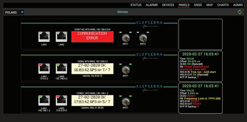
The PANELS is a next MENU item. It groups inside single view window all NTS server virtual front panels. It is simplified version of real NTS front panel. Panels operate real-time (RT) providing all LED/LCD information. Additional information, the one as TIME, OFFSET, OCXO/Rb STATUS etc. are provided too.
