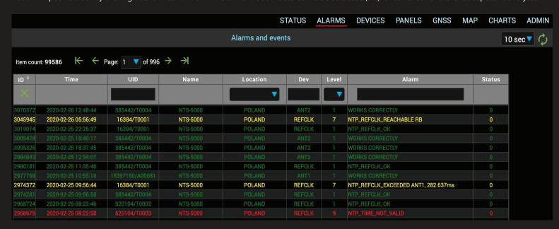
Another way of handling large population of NTS time server devices is text-mode view panel. The special syntactic sugar of this text-mode screen is the right side LED indication row. It provides a real-time device front panel LED status information. Together with other network data it provides general status quo of server group or specific quered it's subgroup.
