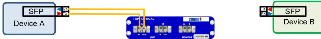
Use same type of cable to connect Port B of TAP to device B
