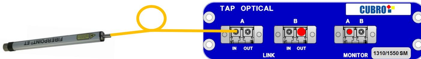
Note: Red light (usually 635 nm or 650 nm) is NOT split in the specified splitting ratio because it is out of the operating window of the splitters! Thus e.g. a 50/50 Multimode TAP might have significant differences in the intensity of the red light at the outputs.
