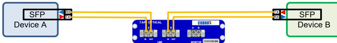
Connect monitoring equipment to Monitoring Ports A and B
