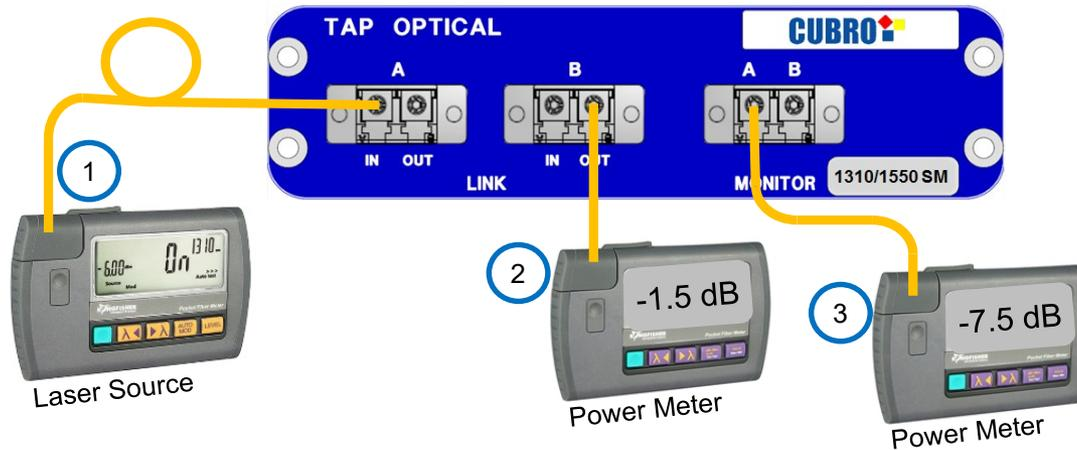
Typical attenuation values including connector loss:
