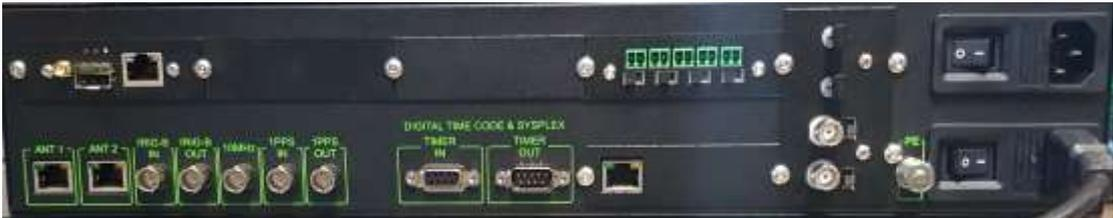
NTS-TC (time-converter PTP-2-IRIG) – back panel view (max. version w/ 4x RS422, 2x FO, 2x BNC TTL 5V AM/DCLS)
