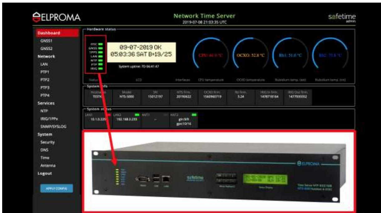
6x LED indicators (from left: OSC, GNSS, PPS, LAN, NTP, PTP, IRIG)
