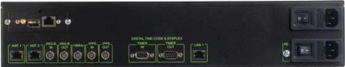
NTS-TC (time-converter PTP-2-IRIG) – back panel view (basic version w/ IRIG-B AM only)
