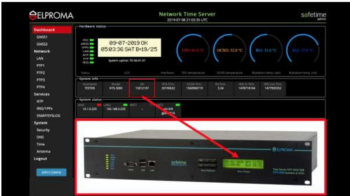
Serial number available on LCD after power-on. Also located on the back-panel S/N sticker
