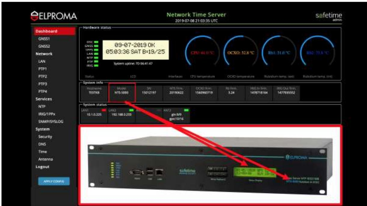
Model (e.g. NTS-5000) available on LCD after power-on. Also located on the right side of front panel
