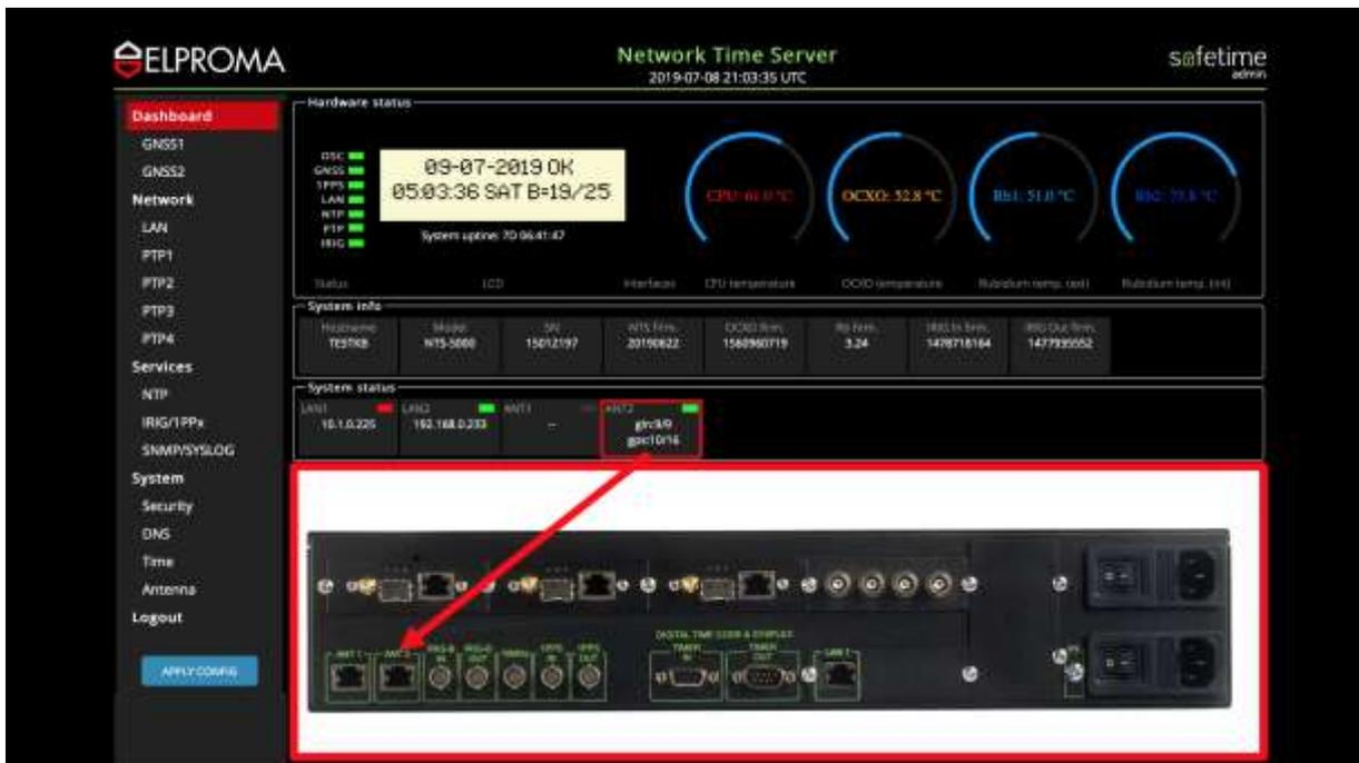
ANT2 back panel LED indicator (blank is NTS-antenna disconnected), and number of SAT is display
