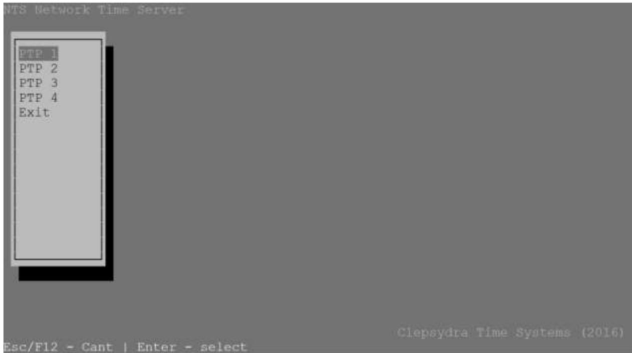
The new setup (different color) screen appears after selecting PTP item from main setup menu. Different color indicates fact that you have entered the security zone of NTS-5000/TC. New menu style includes automatically recognized Expander 1-4 NIC cards. Cards are numbered: PTP1 (Expander 1), PTP2 (Expander 2), PTP3 (Expander 3), PTP4 (Expander 4). Only cards that are recognized by NTS system are displayed.
