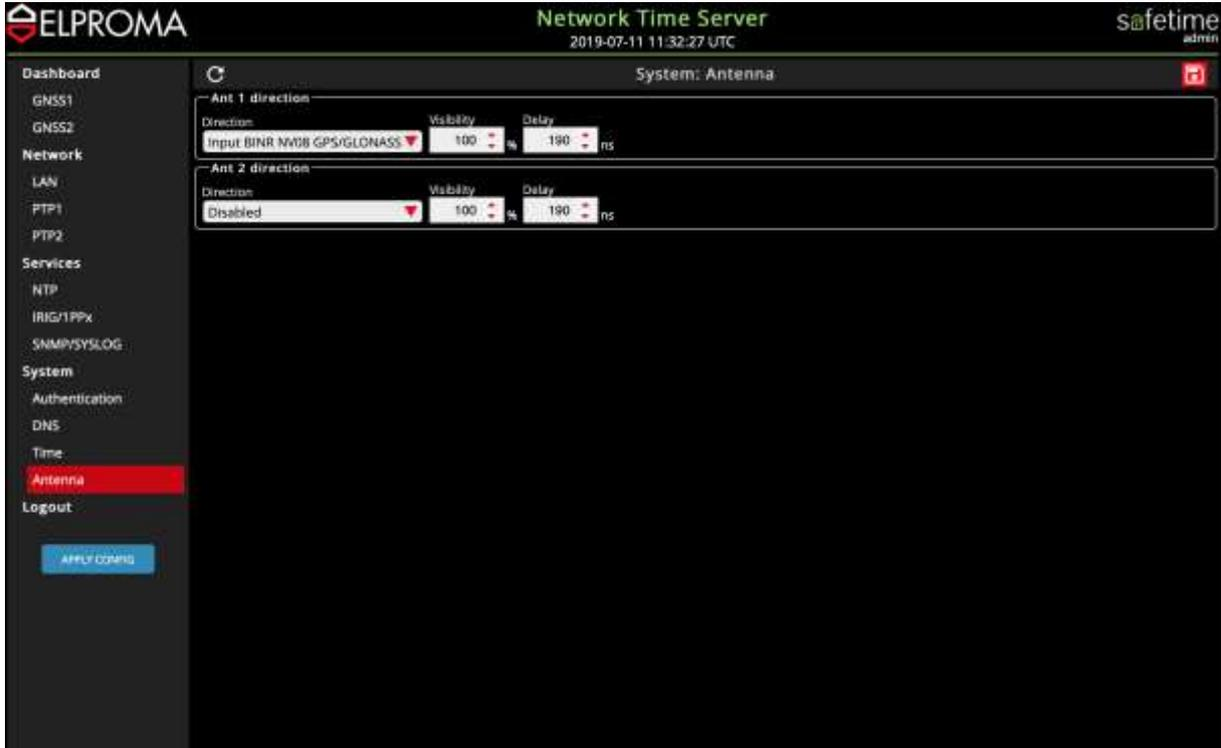
Keeping both antennas enable, when only ANT-1 (or ANT-2) is present, will trigger the front panel GNSS LED flashing RED. This indicates a phantom problem with 2<sup>nd</sup> (not existing) antenna. Please take care to disable not used antenna I/O when only single antenna system is deployed.
