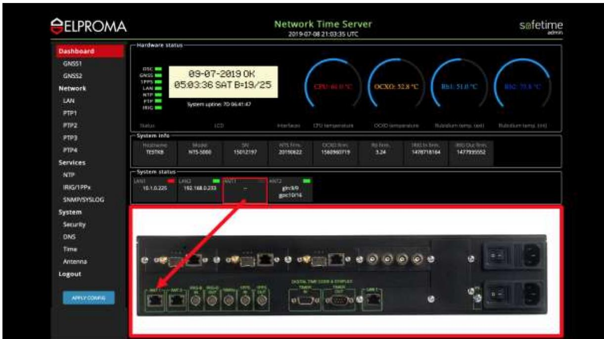
ANT1 back panel LED indicator (blank is NTS-antenna disconnected)
