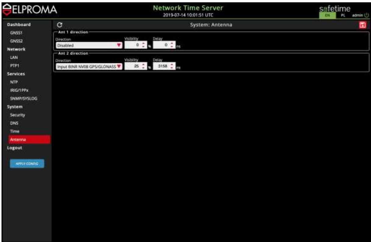
Above example present delay compensation 450ns for 100-meter UTP cat. 5 cable used between NTS-antenna and time server NTS-x000.
