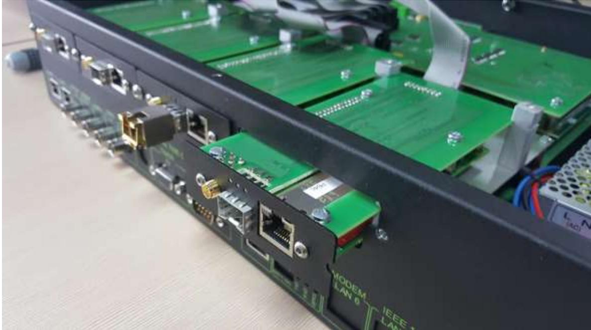
**Expander 1-2 can operate both: grandmaster & slave PTP IEEE1588.** Expander 3-4 are only able to operate as grandmaster. All cards are automatically recognized by NTS-5000/NTS-TC system and added to main menu. Master/Slave is set for all expander, so if you choose to operate Expander1 card slave, both LAN3 and LAN4 will operate slave too. To choose MASTER or SLAVE mode (LAN3-LAN6) select from profile menu:
