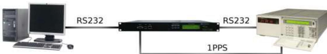
**NOTE!** In Scheme #2 the NTS time server is 100% transparent for PC telemetry dataflow going from/to 5071A via rs232 interface. Typically, PC is used to run Cesium beam monitoring software.
