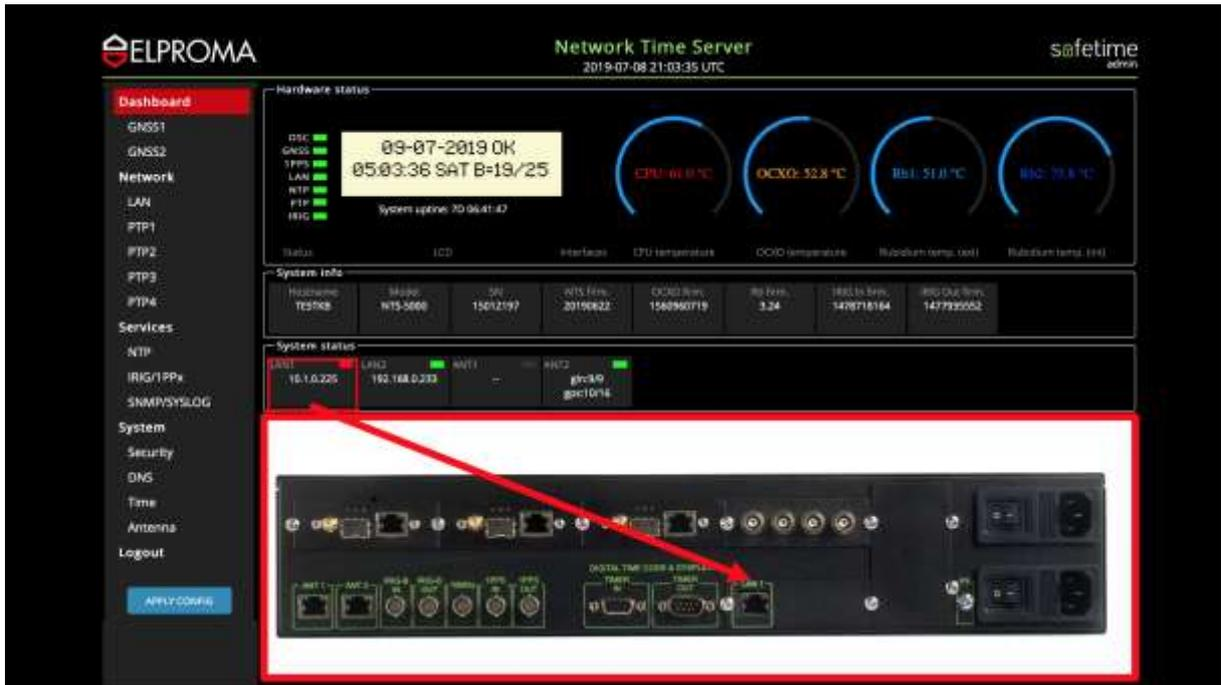
IPv4 address & LAN1 back panel LED indicator (flash red when Ethernet network cable disconnected)
