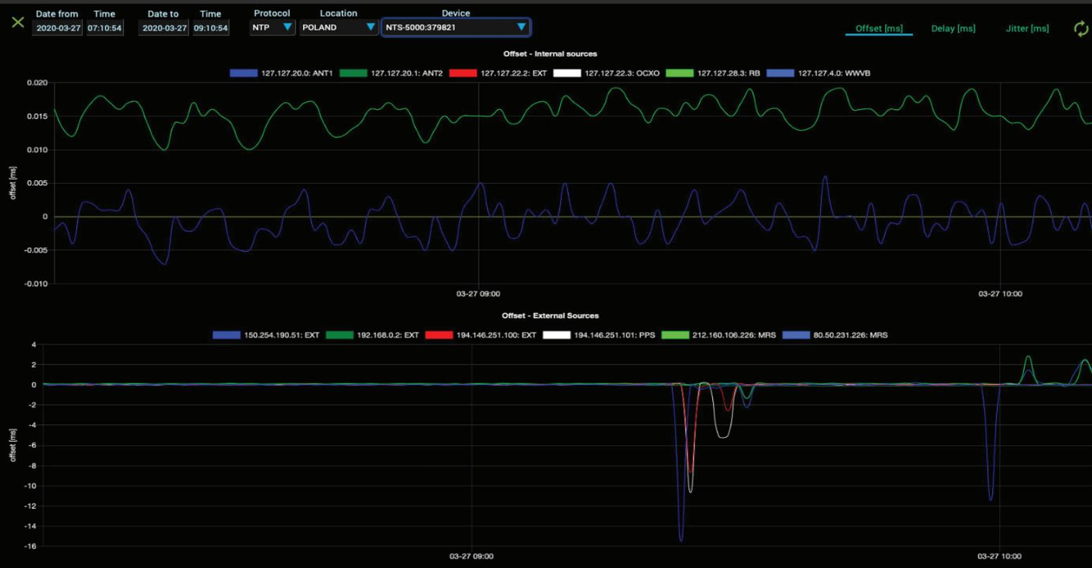
Plotting charts is one of major functionalities. Multiple servers can be observed simultaneously for all 3 parameters: OFFSET to UTC, network DELAY, synchronization JITTER. It lets administrator compare beehive of time servers located in different places but measured from one common point of reference – the central management system.
