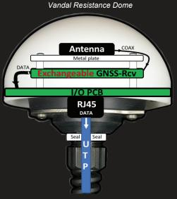
Single smart NTS-antenna is included to NTS-3000/4000/5000/LITE time server at arrival. Redundant 2nd antenna\* is optional. It improves security and robustness of synchronization. Compering to other products, the smart NTS-antenna has built-in modular GNSS receivers. Replaceable GNSS receiver can be supported by different CHIPS, from different vendors:
