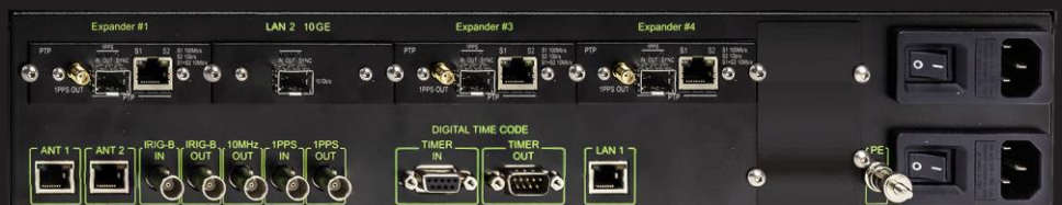
DATAKOM9: 6x1GbE LAN3-8 (Hardware Time-Stamping) + DATAKOM2”(LAN2)
