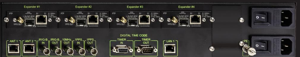
DATAKOM7: 8x1GbE LAN3-LAN10 (Hardware Time-Stamping) + DATAKOM1
