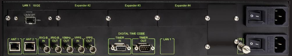
DATAKOM2: 1x10GbE(LAN1) + 1x100/10Mbps LAN2 (Software Time-Stamping)
