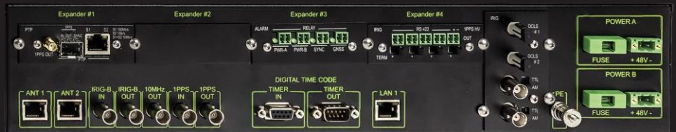
SMART-GRIDS CUSTOM1 – This is PTP SLAVE generating IRIG like SMARTGRIDS4
