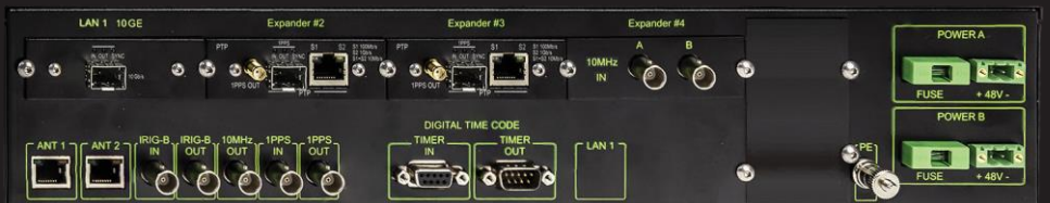
TELECOM-9 ePRTC 1x10GbE, 4xGbE HW-stamping Autonomous GrandMasters
