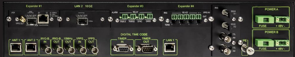
SMART-GRIDS CUSTOM2 – This is PTP SLAVE + CUSTOMS1 (above) + 10GbE out
