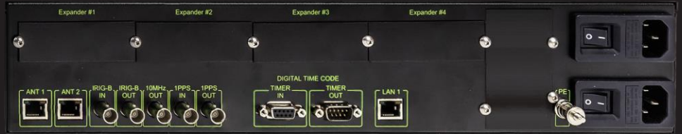
DATAKOM1: 2x100/10Mbps (Software Time-Stamping) LAN1&LAN2
